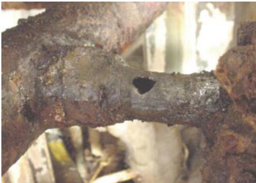
Figure 2: Typical corrosion under insulation
